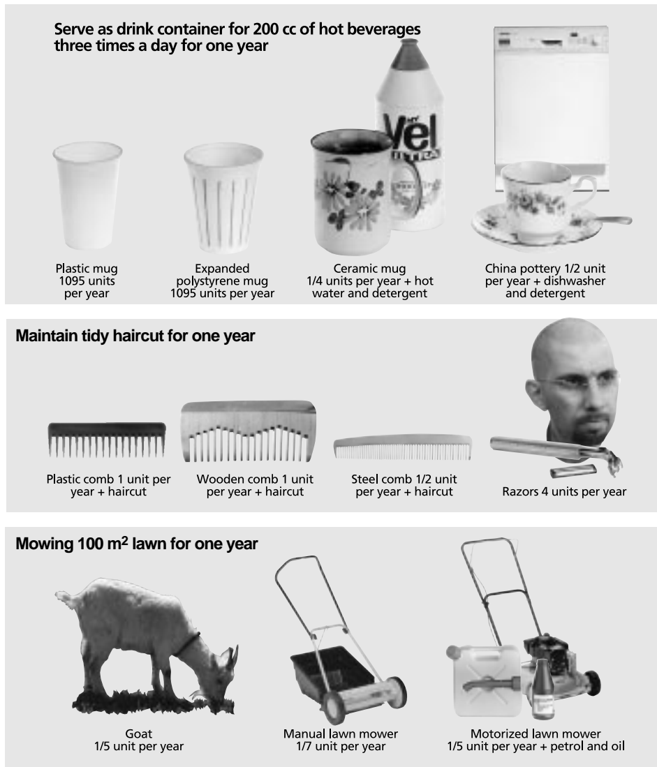
Figure 4. Different ways of obtaining the same functional units (Wenzel et al. 1997).
